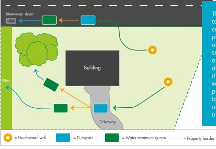
The colored groundwater is pumped to the dumpster where the stone cuttings sink to the bottom. The purified water is then pumped out on your land and absorbed by the soil. If it is not possible to pump out the water on your yard, we direct it outside the boundaries of the property, e.g. to a ditch or a woodland. The water can also be pumped to a stormwater drain as long as it is first filtered through our RotoCont or RotoCont+ water treatment system.
